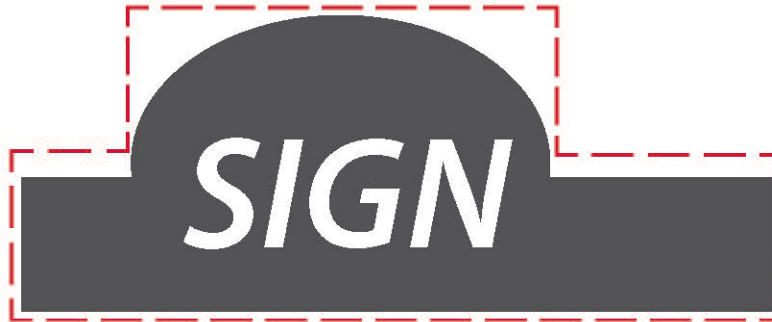
Figure VIII-1. Measurement of Sign Can, Cabinet or Frame
