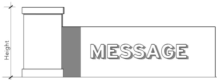
Figure VIII-4. Measurement of Sign Height
