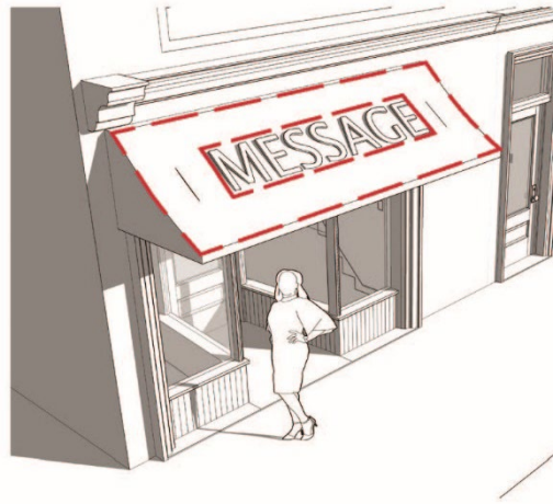
Figure VIII-3. Awning and Canopy Sign Measurement
