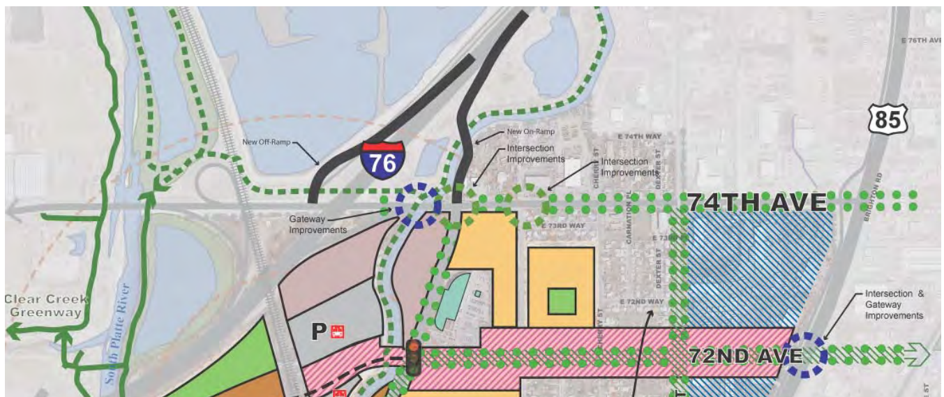
Proposed circulation improvements on and off I-76 at 74th Avenue will provide greater access to the station and future development
