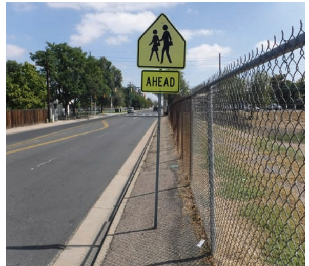
Pedestrian Barrier Resulting in Vehicle Conflict
