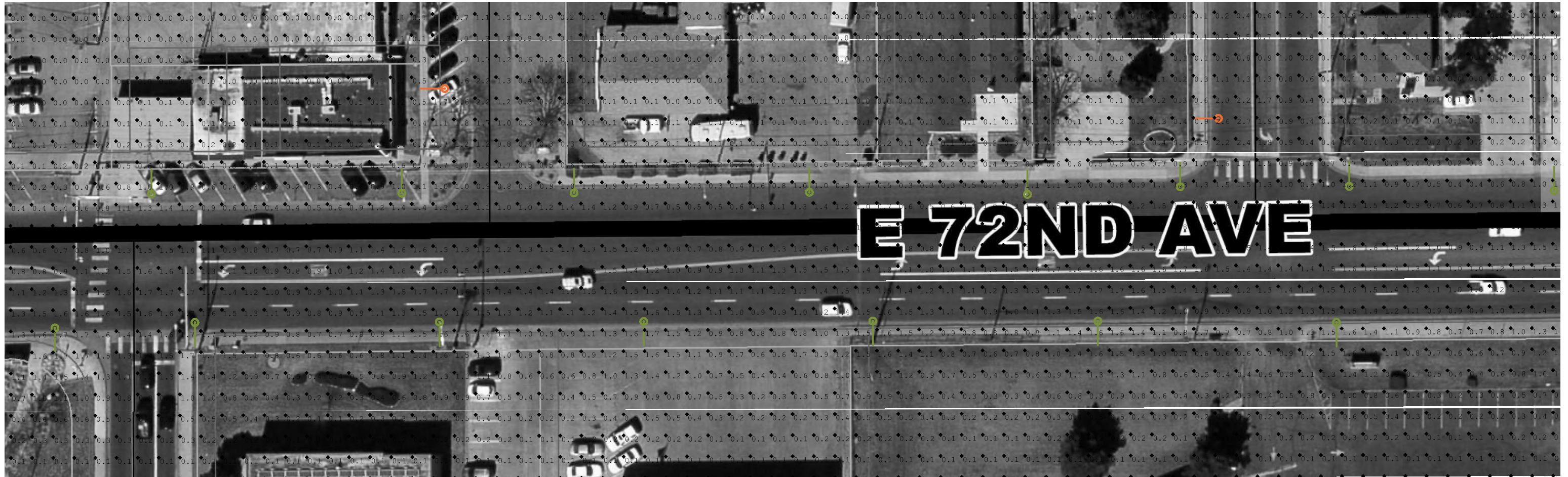
Depiction of photometric calculations that represent achievable light levels when fixtures are spaced according to the specified design guidelines.
