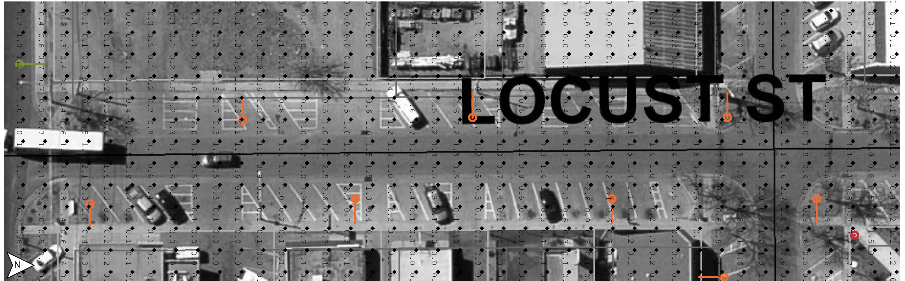
Depiction of photometric calculations that represent achievable light levels when fixtures are spaced according to the specified design guidelines.
