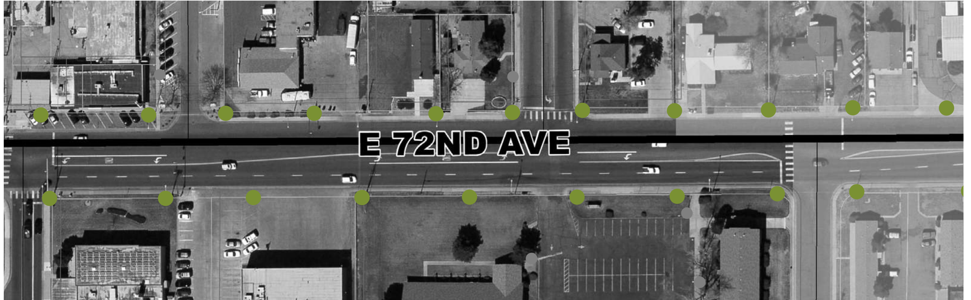
Map of the recommended light fixture spacing for large collector roadways.
